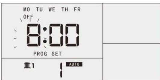
Press [SELECT] to set Channel 1 Weekday P2-ON. Press [UP] or [DOWN] to set hour. Then press [SELECT] and press [UP] or [DOWN] to set minute.
