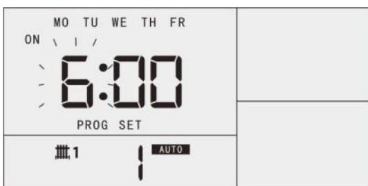
Press [SELECT] to set Channel 1 Weekday P1-OFF. Press [UP] or [DOWN] to set hour. Then press [SELECT] and press [UP] or [DOWN] to set minute.
