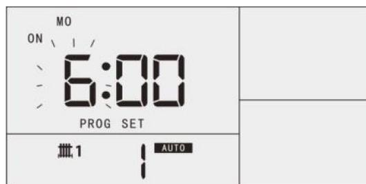
Press [SELECT] to set Channel 1 Monday P1-OFF. Press [UP] or [DOWN] to set hour. Then press [SELECT] and press [UP] or [DOWN] to set minute.
