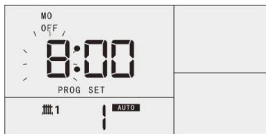
Press [SELECT] to set Channel 1 Monday P2-ON. Press [UP] or [DOWN] to set hour. Then press [SELECT] and press [UP] or [DOWN] to set minute.
