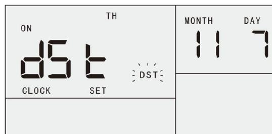
Daylight saving time is set to ON
