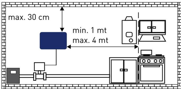
METHANE is a gas lighter than air, the maximum concentration is located near the ceiling. Install the unit on the wall, about 30 cm from the ceiling and at a distance from gas using device, between a minimum of 1 meter and a maximum of 4 meters.
