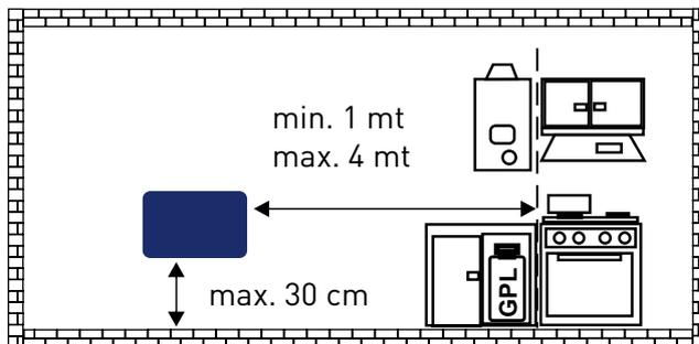
LPG is a gas heavier than air; the maximum concentration is located near the floor. Install the unit approximately 2 meters (minimum 1m, maximum 4m) from the gas using device and about 30 cm from the floor.
