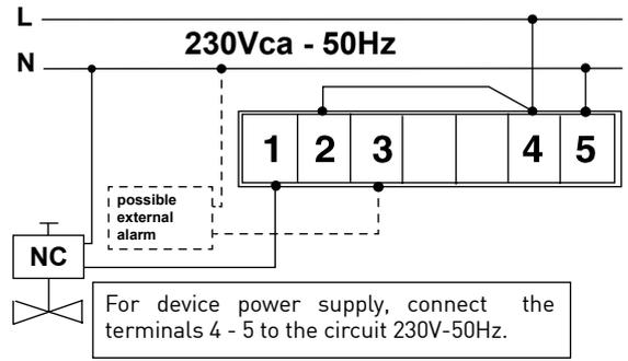
EXAMPLE OF CONNECTION of Sicurgas P11 with IMPULSE RELAY, with current activation, to control a normally open NO valve with manual reset (switch in up position).
