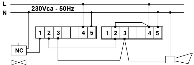
Example of connection for several Sicurgas detectors with impulse relay, which control the same normally open valve NA.
