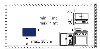
LPG is a gas heavier than air; the maximum concentration is located near the floor.
