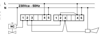
Example of connection for several Sicurgas detectors with impulse relay, which control the **N** same normally open valve NA.
