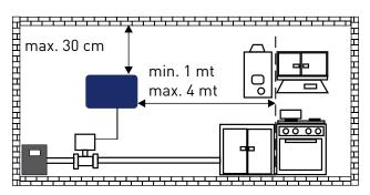
METHANE is a gas lighter than air, the maximum concentration is located near the ceiling.
