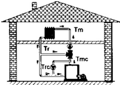
**3-WAY ROTOR POWER-OPERATED MIXING VALVE**
