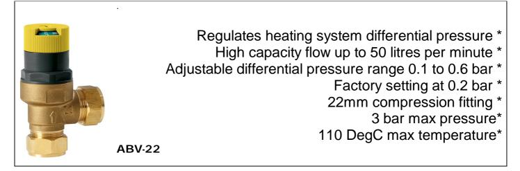
The Banico ABV should be fitted where a boiler bypass is required – typically this is the case when a system is equipped with thermostatic radiator valve, and to allow pump over run operation after zone valves have closed down
