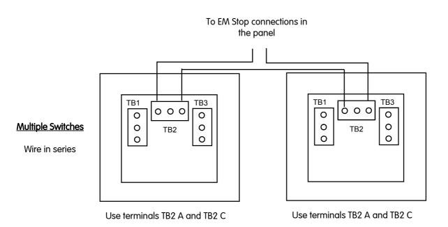
Remote stop buttons can be connected to the panel terminal marked as "EM STOP" (number 6). The remote buttons must be wired as above in order to provide a "closed contact" for the control panel.
