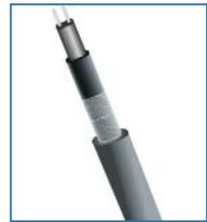
Conductor section 0,57 mm 2 Self-regulating conductive core Polyolefin sheath Copper braid Polyolefin external sheath
