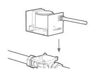
**6-** Replace the cover and screw. Release lever and allow to travel back to "AUTO".
