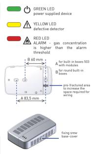
After executing the mounting and the connections (see paragraph 4) replace the cover on the base ensuring the two cover pegs are correctly located on the two latching tabs. Screw again the fixing screw and apply in the corresponding place the provided adhesive label indicating the replacement date.
